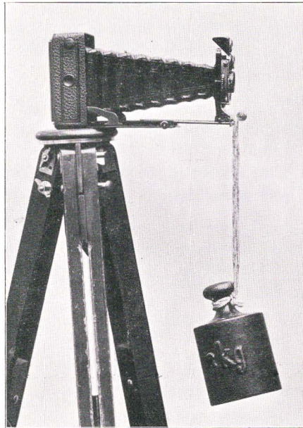
Severe Test of the "Tourist" Vest Pocket Camera, loaded at full extension with a weight of 2 kg (4 lbs. 6 \frac{1}{2} oz.)
