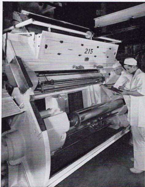
Photographic film base emerging from a roll-coating machine. This is the "windup."
