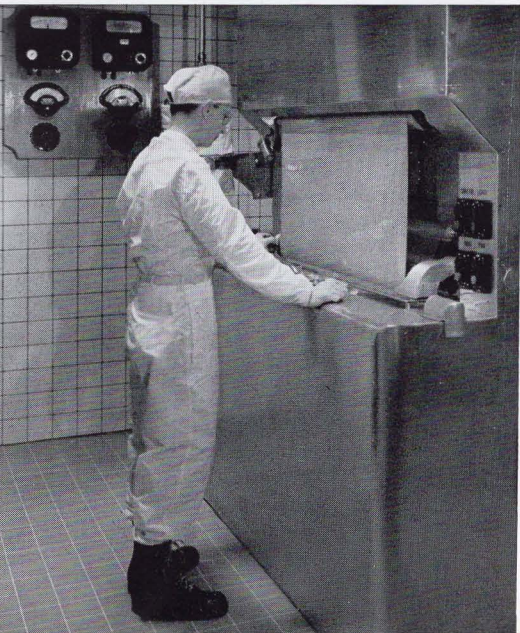
Photographic film base emerging from a roll-coating machine. This is the "windup."
