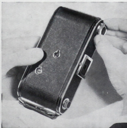
Winding the film for 8 exposures. Two ruby windows are fitted, one for 8 and the other for 12 exposures. The respective numbers are clearly marked on the sliding covers.
