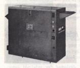
†Kodak Versamat Film Processor, Model 11A-M—For rapid, automatic, and controlled processing and drying of 4x5 through 11x14 black-and-white sheet films. With available accessories, listed below, accommodates continuous lengths of 16mm through 9½-inch-wide roll film. Stainless-steel consistent and temperature control of solutions (at least 4 gallons per min-
