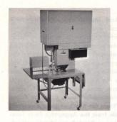
†Kodak Roll Paper Printer, Type IVB-3 (5x7) — Extremely versatile high-speed roll paper printer for making any size prints up to 7 inches long on roll paper up to 5 inches wide from any negative size up to 3½x5 inches. Ideal for "school," "wallet," and identification pictures, in black-and-white or color, using single or multiple lenses. Also readily adaptable to black-and-white 5x7-inch enlargements and 4¼- or 3½-inch greeting cards from photofinishing negatives.
