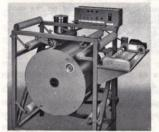
†Kodak Roll Paper Dryer-Glazer, Model C-2—A compact, versatile ferrotyping dryer for black-and-white or color papers, after processing in various Kodak Continuous Paper Processors. It can, however, be threaded for either matte or ferrotyping use. Capacity up to 6½ feet per minute. Highly polished, chrome-plated drum can be easily removed and replaced.
