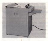
†Kodak Master Roll Paper Holder, Model 11-K—For rapid production of enlargements in roll form up to maximum size of 11x14 inches with a maximum paper width of 11 inches. The paper is advanced on a flat printing surface under a wall-mounted or table-mounted enlarger. Available accessories are the Kodak Pencil Marker, Model 6, and Kodak Print-Cutting Pencil Marker Bracket, Type MRH (for
