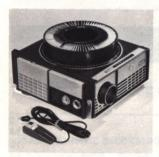
Design—A round, 80-slide tray is positioned on top of the projector, and simple gravity feed drops the slides into projection position. This unique system offers jamproof operation, longer one-tray slide shows, and the advantage of continuous operation for display and advertising. Controls for automatic operation, slide changing, and focusing are provided at the projector. Full remote control of slide change and focus is afforded by a 12-foot remote control cord. The
