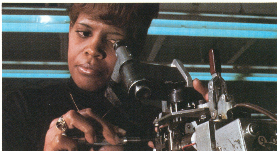
Skilled worker performs a rangefinder adjustment on a Kodak XL movie camera.
