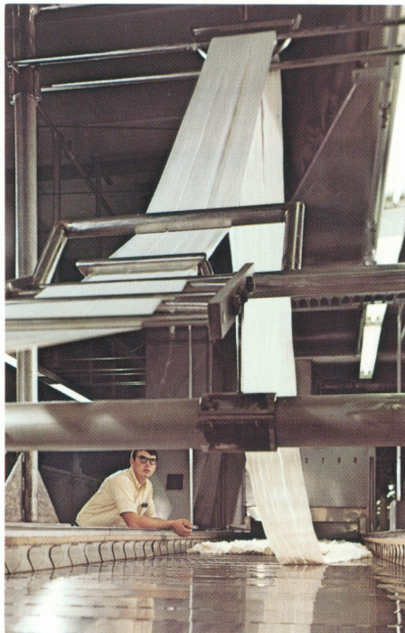
Strands of Kodel polyester fiber travel through dryers before being cut to staple lengths at Carolina Eastman.
