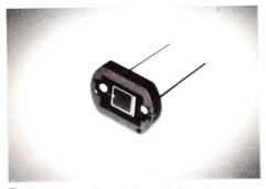
Fast response silicon photo diode adjusts quickly to abrupt light changes.
