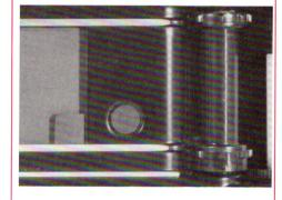
A film blind inside the camera lowers to block the recording area.
