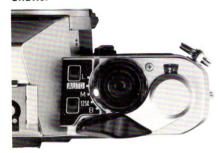
Seiko MFC-E2 vertical-run metal focal plane shutter; automatic exposure electronically controlled in stepless range from 4 seconds to 1/2000 second; full range of 14 manual shutter speed electronically timed from 4 seconds to 1/2000 second, controlled by dual pushbutton action; mechanical speeds of 1/125 second and B operational without batteries; shutter release lock provided; 5 position shutter mode selector.
