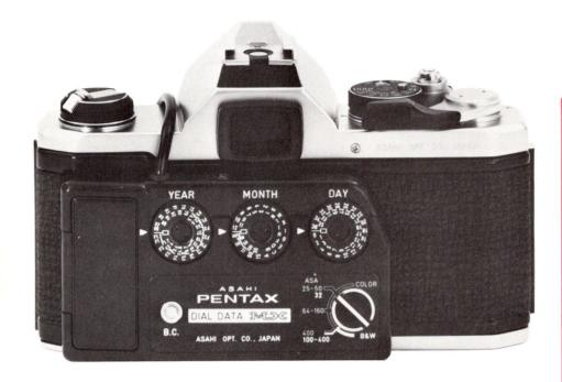
The Dial Data MX can be set to record the date (day, month, year) the aperture, shutter speed and frame number, or an alphanumerical code selected by the user, in the lower left corner of the (horizontal) photograph or transparency.
