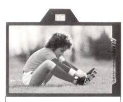
The Viable Viewfinder. In the above example, the following information is available at a glance: The aperture is f/5.6, no compensation is being used, the camera is set to AUTO, the automatic exposure is approximately 1/125, and the subject is properly composed and focused.
