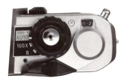
Seiko MFC vertical-run metal focal plane shutter; automatic exposure electronically controlled in stepless range from 1 second to 1/1000 second; mechanical speeds of 1/100 second and B operational without batteries; 3 position shutter mode selector.
