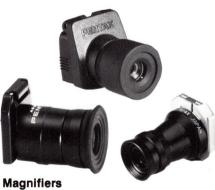
Easily clips on to the grooves of the eyepiece to magnify the central portion of the focusing screen 2X for critical focusing. The hinged magnifier can be raised to view the entire focusing screen, and it has a built-in eyepiece correction lens with an adjustable diopter range.
