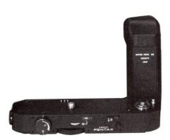
The powerful micro motor of the compact Motor Drive MD, the heart of the K2DMD motor drive system, propels the film at a rate of  $\frac{1}{2}$ -2 fps. Furthermore, a single touch is all that is required to changeover from single-frame to consecutive exposure operation. Also found on this unit are the exposure counter, trigger release, remote control socket, tripod socket, and rewind lever.
