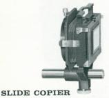
Here is a real copying ease for duplicating slides. Slide stage raises or lowers for precise positioning, and a separate set of bellows shuts out all light between the slide and the lens, preventing lens flare from the light source. Used with Bellows Unit II.
