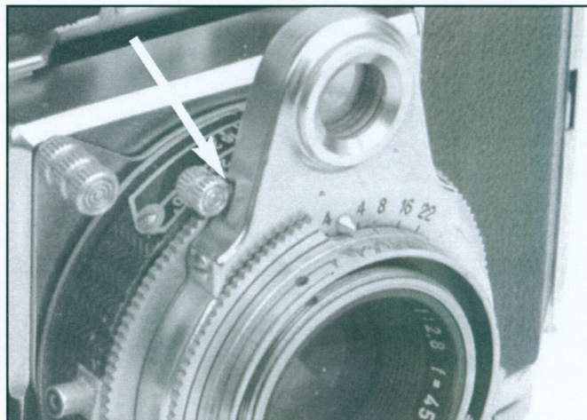
The shutter-cocking lever shown in the un-cocked position (left) and fully cocked (right). The arrow in the left-hand view shows that the small knob on the end of the lever has had much of its width milled away. When fully cocked, even with this modification the knob can only fit properly against the rangefinder-prism housing when a small slot (arrow) is cut into it. Figure 7
