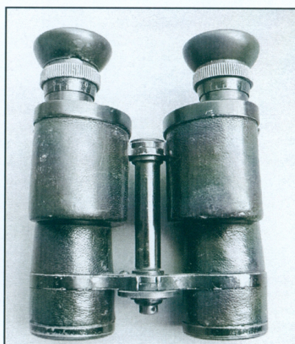
The Goerz 6×30 Pernox, a dustproof model that did not need to be cleaned in the field. The one shown here is serial number 59769 from 1904. Figure 8
