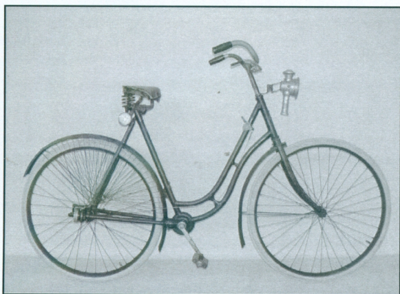
A shaft-driven bicycle. This 1910 lady's model Durkopp is similar to the slightly earlier gentleman's bicycle shown in our photograph of Rudolph, Abbe and Schott on page 4 of the Fall 2009 issue. I mistakenly assumed that the bicycle had lost its chain, but Peter von Thuna has corrected me, above.
