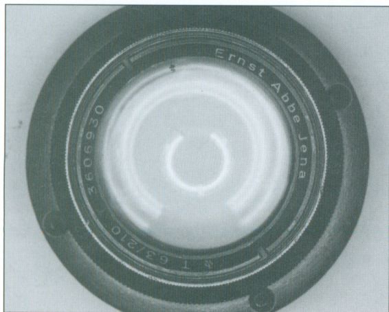
A "Carl Zeiss" Tessar with an "Ernst Abbe" identification
