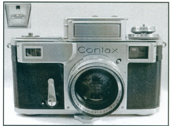
An unfinished CZJ Contax III lacking a meter/rewind assembly, a winding knob, and a serial number in the flash shoe (insert in upper left corner). Moreover, the lens ring is not painted in black with white lettering and numbering, rather it is black on a metal background.
