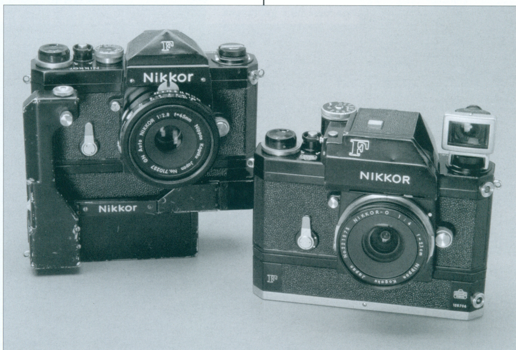
On the left, a 'Nikkor' F camera with eye-level finder and an F36 'Nikkor' motor drive from batch #9. On the right, a 'NIKKOR' F with an extremely rare 'NIKKOR' Photomic T finder Type 2R and an F36 Nikkor motor drive from batch #1.
