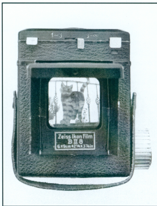
The photographer's view shows the 35 \times 35 mm brilliant finder, the shutter release and settings located at the two front corners, and the close-up lever between them. Figure 6
