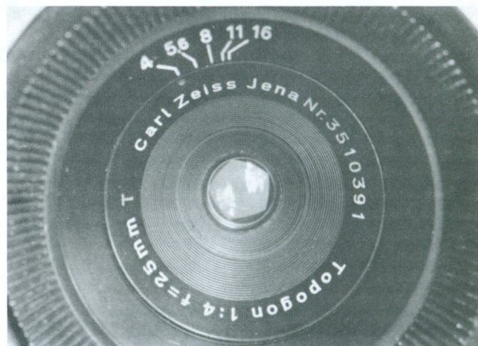
Prewar Topogon f4.5 (top) with diaphragm at widest aperture. Note how much smaller this is than the largest possible opening. This, like the smallest opening (f11), was presumably for flare control. Postwar Topogon (bottom) opens to f4, closes to f16 — an increased range that results from T-coating.
