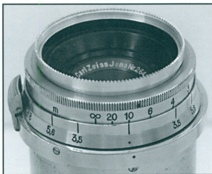
Depth-of-field scales on the three 3.5cm lenses shown on page 13. Left to right Orthometar, Herar, Biotar. Photos: Barringer
