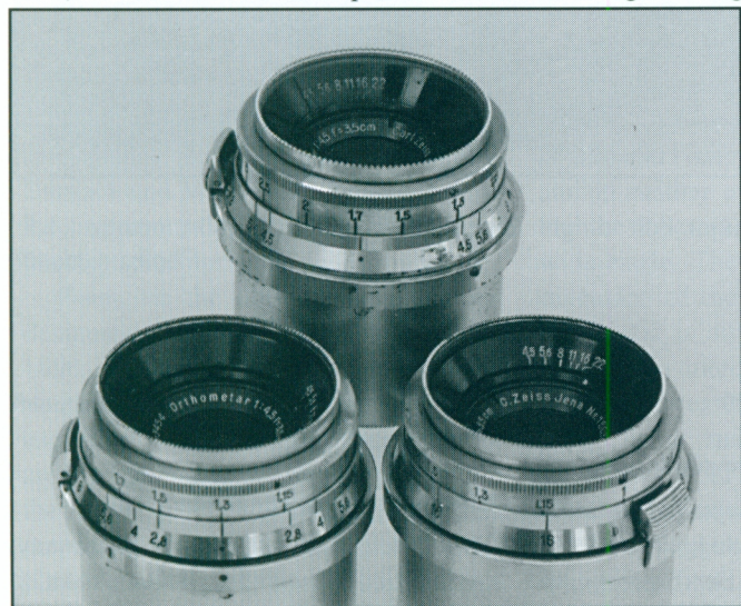
Detail of Orthometar variations. Clockwise from rear: Normal configuration; preproduction version marked "C. Zeiss Jena"; early version in Biogon mount with "f: 2.8" marking on depth-of-field scale. Photo: Barringer
