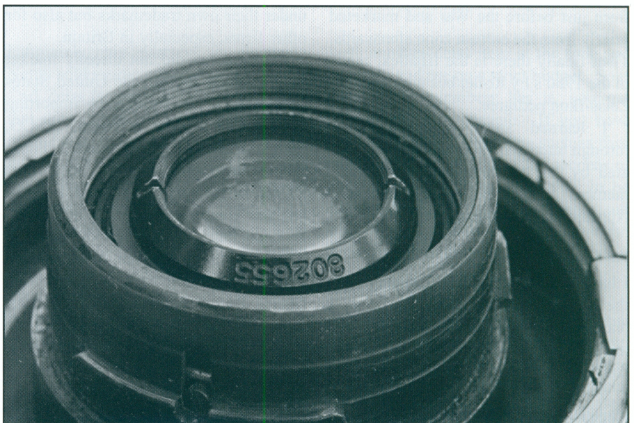
Rear view of a Biotar 3.5cm f : 2, showing the engraved six-digit number. Most Zeiss lenses, like this one, have a rear number that lacks only the "millions" digit of the full serial number. Photo: Barringer
