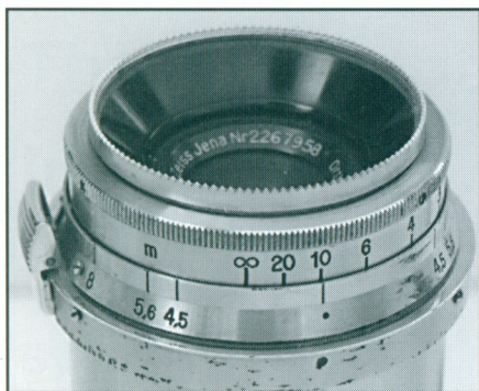
Depth-of-field scales on the three 3.5cm lenses shown on page 13. Left to right Orthometar, Herar, Biotar. Photos: Barringer
