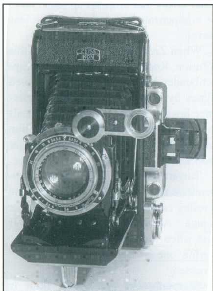
Super Ikonta C , one of the cameras that used the rangefinder design of the Contax in a format originally more commercially successful than 35mm.
