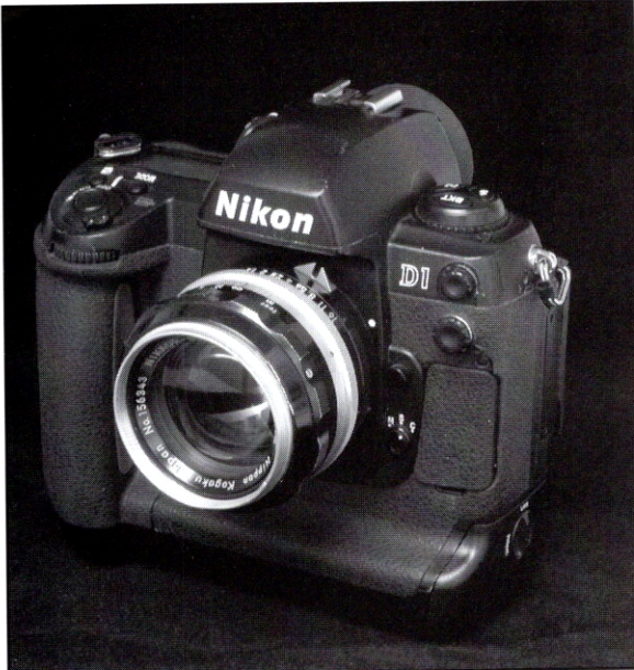
Above..Nikon D1 from July 1999 plus Nikon 5.8cm/f1.4 from March 1960 mounted. Nearly 40 years apart & still compatible! Right..Nikon D1 + box + Battery EN-4 + AC adapter EH-4 + MH-17 auto (12V) battery adapter (MH-16 battery adapter came with camera) + D1 focusing screen E.
