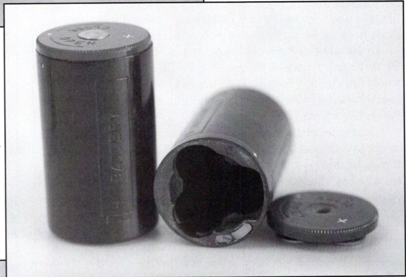
Above & above right..An original 25V 'Power Unit for BCB' mentioned in the text. Note the three top contacts, the protruding coil spring & the grounding spring going down the side, all of whose functions are explained in this article. Right... Two examples of the 2nd type battery holder designed for three AA-size penlight batteries. Modern AAs are slightly longer than those from the 50's and do not fit. However, Jeff tells me that a smart tap to the contact nipple on the battery top shortens them just enough. Below.. Two examples of the black plastic 'battery holder' for the rectangular hearing aid type battery and the AA-size capacitor.
